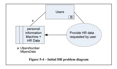
Figure 5-4 shows the problem diagram for the requirement and context. There are two phenomena of interest. The first, U!persNumber, is the user's request for personnel information. The second, M!persData, is the information returned by the request.
