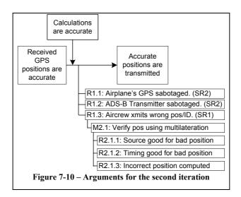
create 'virtual transmitters' at any position (Capkun & Hubaux, 2004). The third rebuttal (R2.1.3) challenges the assumption that the clocks in the receivers are synchronized. It is possible to perturb the clock at particular receivers, which would cause the position calculation to be offset. More detail on this rebuttal would require looking at specific multilateration time synchronization solutions.
