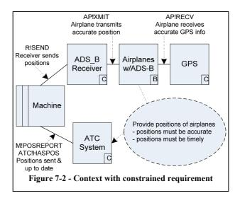
The NATS requirement for accuracy is that the aircraft be within 300 meters of its reported position when the position is received. However, ADS-B can potentially improve on that by an order of magnitude, and the consequences of this must be studied. SR1 operationalizes SG1.
